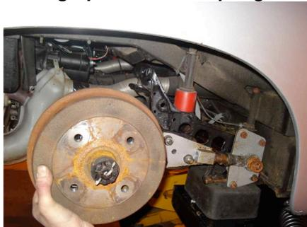
A small amount of camber adjustment should also be available. This is normally achieved by using an eccentric / slot on the foremost spring plate bolt. Adjustment would allow for synchronisation of the camber across the rear axle which should be less than 30minutes of a degree for fine handling (removal of camber thrust effect).
