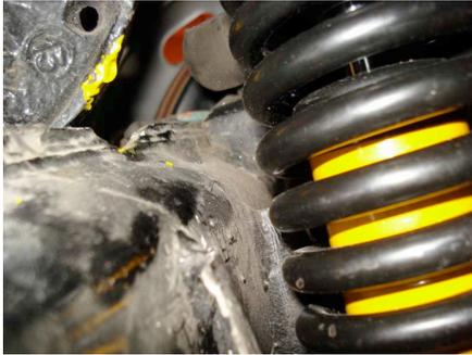
Original factory cars running ride heights of 260mm at the rear are not known to have shown this problem. This may be due to a combination of COFAP damper /spring and factory rubber bump stop and slightly higher ride heights.
