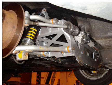
Despite the further ride height increase, the offside rear trailing arm still hits the chassis on high speed bump. Either the extra driver weight or differing tolerances of chassis/arm are suspected to be the reason.
