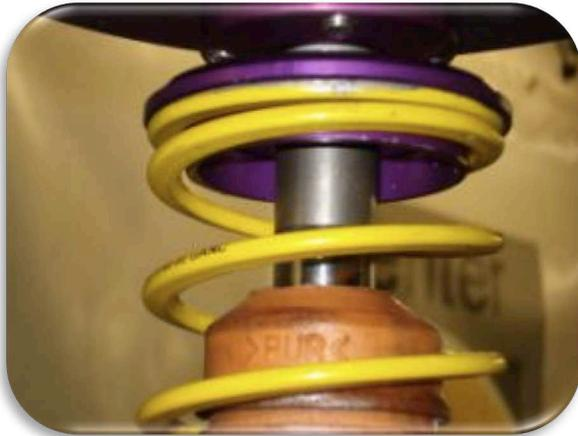
Fig 3. 20mm spacer tube fitted on 993RS damper rod for correct top mount position for C2
