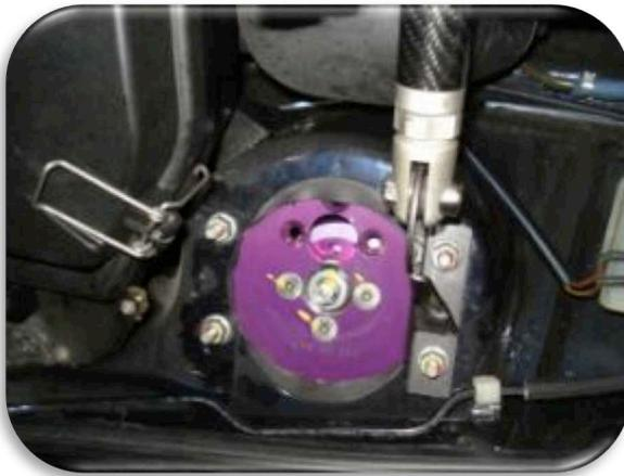
Fig 5. Modified top mount installed to give 0 to 2degrees negative camber
