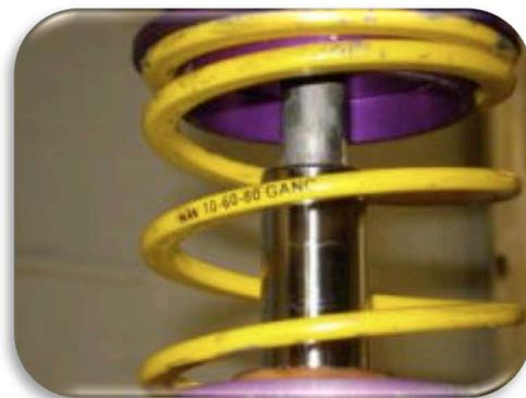
Fig 2. Shoulder of 993RS damper rod too short for top mount / fitting to 993 C2 prior to spacer being fitted
